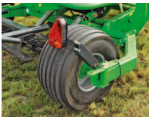
During road transport, the right-hand wheel can be folded inward
