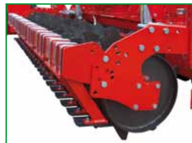
Rullo packer (Ø 406-464-500-550) GB Packer roller F Rouleau packer D Zahnpackerwalze E Rodillo packer
