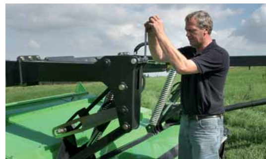
The cutting height is set by turning an integrated handle on top of the suspension.
