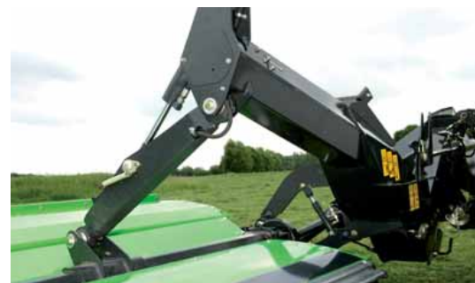
Pulled centre suspension for even weight distribution and excellent adaptation.
