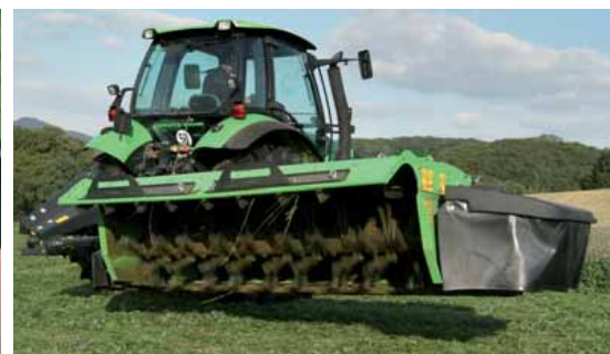
Easy lift on headlands without activating the 3-point linkage of the tractor.
