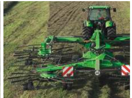
The two outer rotors can be adjusted individually to match a working width between 9.50 m - 15.00 m
