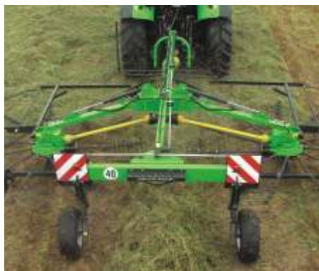
SwatMaster 7041 with 7.00 m working width
