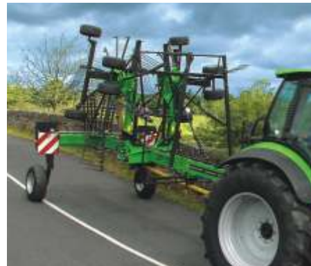
Deutz-Fahr centre swath rakes are converted hydraulically for transport from the tractor cab. To limit transport height further, the main frame can be lowered hydraulically as an option and the tine arms can be removed.
