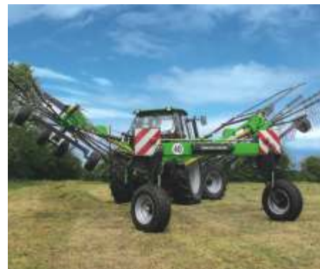
The high-clearance frame gives up to 45 cm lift-out to safely pass over swaths during headland turns.
