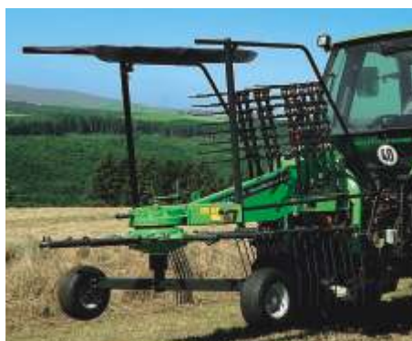
All rakes can be set to narrow transport width by removing the tine arms and placing them on the carrier frame
