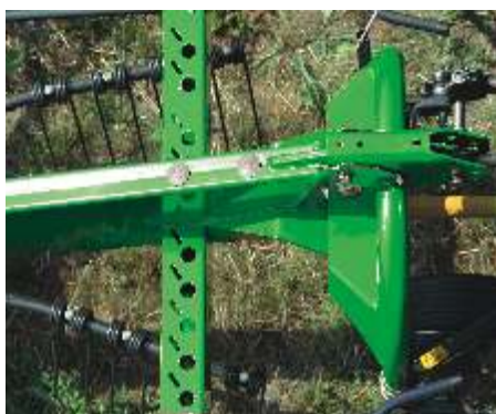
A pivoting 3-point headstock ensures perfect ground following performance and perfect tracking when cornering
