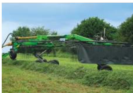
With 50 cm lifting height, swaths can be run over with no problem at all. Rotors are lifted using only a single acting valve
