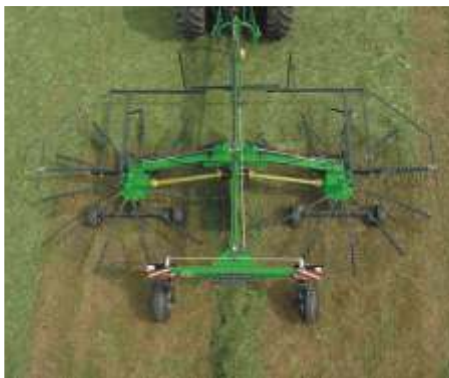
The setting system allows swath widths from 1.20 m to 1.90 m to suit for any pickup system and any forage system - baler, forage harvester or forage wagon.
