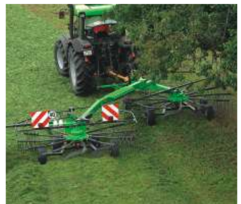
SideShift to the left – raking without running on unraked crop
