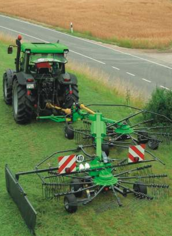
The SwatMaster 7131 featuring 7.10 m working width and unique new SideShift device
