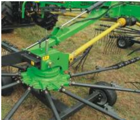
The rotors can be set hydraulically from 7.00 m to 7.80 m working width
