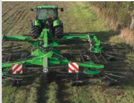
The two outer rotors can be adjusted individually to match a working width between 9.50 m - 15.00 m
