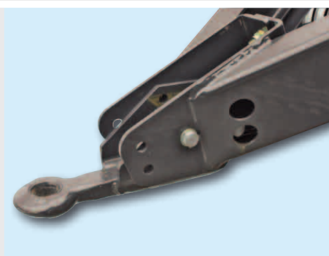
Several hitch options and a reversible drawbar
