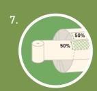
There should be an overlap of at least 50% and 4 to 6 layers of film applied.
