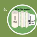
The film must be wrapped around the bale with a prestretch percentage which is between 55% and 70%.
