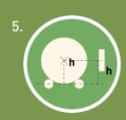
The pre-stretch unit must be positioned in such a way that the middle of the ®Silotite reel is placed at the same height as the middle of the bale.
