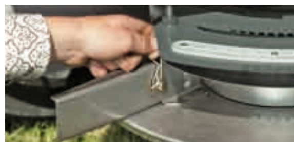
4 detachable vanes per disc determine the working width
