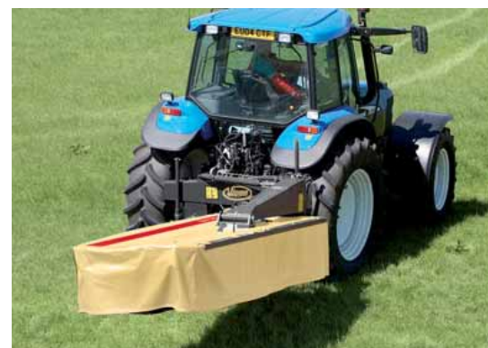
The mower is swung hydraulically into a horizontal transport position.
