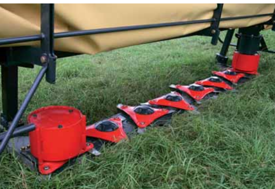
The complete front can be opened for easy inspection of the cutterbar.
