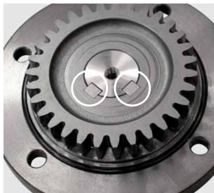
To protect the gear wheels and the drive system, Vicon uses a two-key safety device, designed to break in case of overload.
