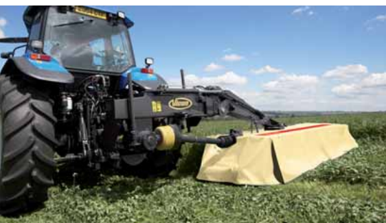
Hydraulic suspension for precise setting of ground pressure.
