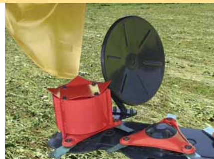
Swath disc (optional) to separate the mown crop from the unmown.
