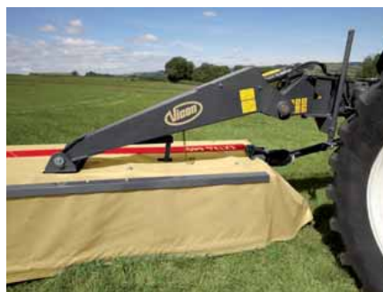
Centre suspension for even weight distribution.
