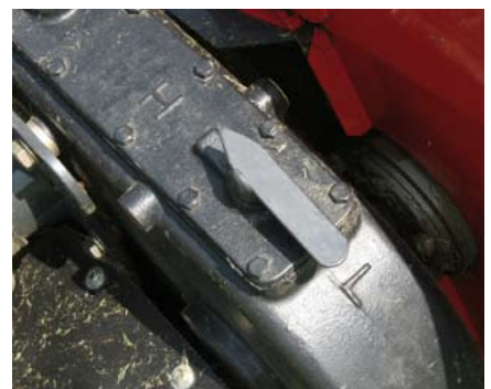
Conditioner speed of 900 or 600 rpm - changed in a second.
