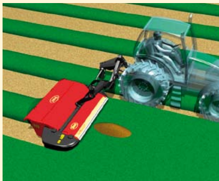
If an obstacle is hit in the field the pulled suspension allows the mowing unit to swing backwards and up.
