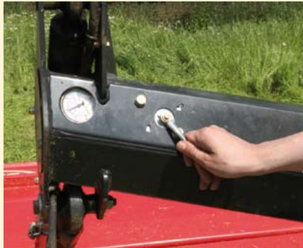
Hydraulic suspension for easy and precise setting of ground pressure.
