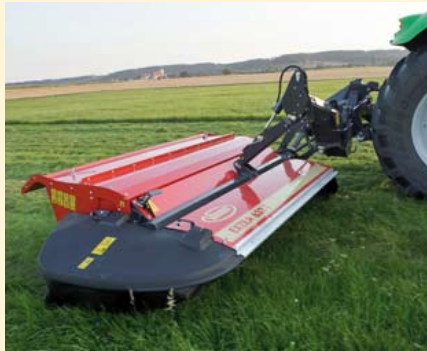
Pulled centre suspension for even weight distribution and excellent adaptation.
