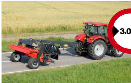
Narrow transport width of 3.00 m of the EXTRA 832 Pro versions and 3.40 m for the EXTRA 835 Pro versions.
