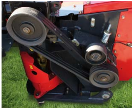
The conditioner's V-belt drive with easy switch of pulleys. Switch the pulleys to change the conditioner speed from 600 to 900 rpm.
