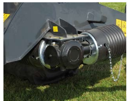
540/1000 rpm adjustable gearbox as standard.
