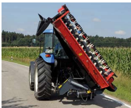
EXTRA 624T and 628T are folded into a 125° vertical transport position using a hydraulic cylinder.
