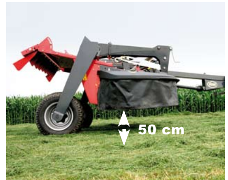
The high-lift design of the mower gives a lifting height of 50 cm. The result is good clearance for transport and when turning on headlands so that swath damages are minimised.
