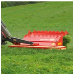
Individual lift of each mower unit.
