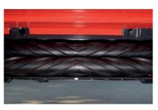
Conditioning intensity is varied by adjusting the minimum gap between the two rollers. Both rollers are driven.
