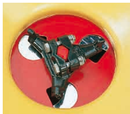
Agitator ensures even feed of the fertilizer
