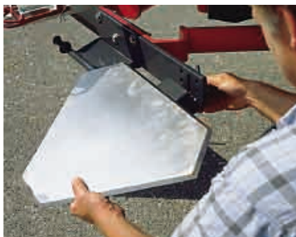
Quick fitting of deflector plates for 18m spreading width
