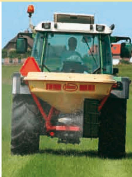
Border spreading with the border spreading plate
