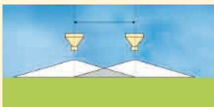
The cone shaped spreading pattern reaches from tractor wheel track to tractor wheel track giving total overlap of the spreading surface
