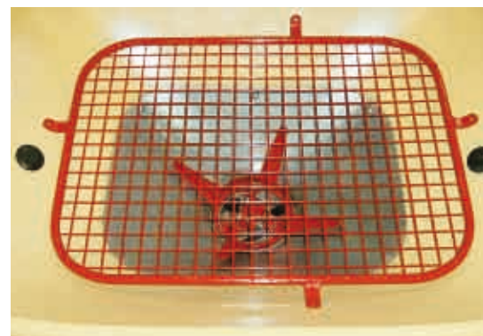
Agitator with safety grid
