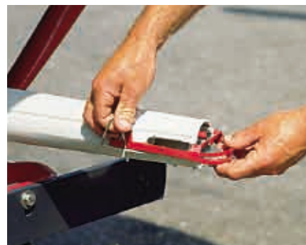
Spout band for 18m spreading width
