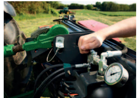
Hydraulic setting of ground pressure (EXTRA 428H & 432H).
