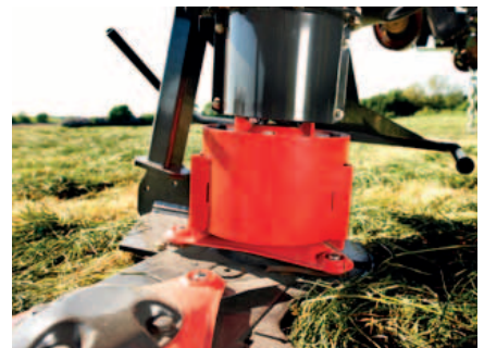
Direct drive from the gearbox to the first disc for efficient power transmission.
