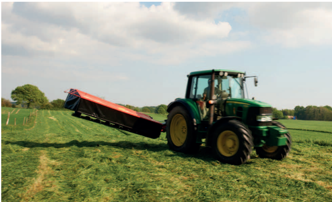
Lifting on headlands via a hydraulic cylinder.
