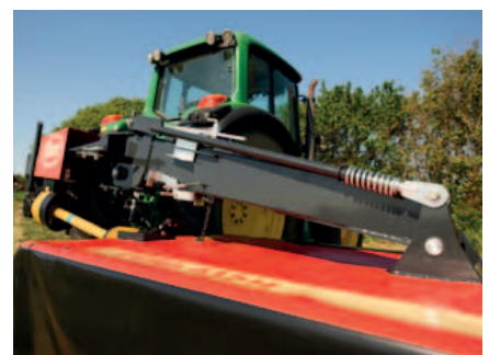
Any ground-unevenness is absorbed by the suspension.
