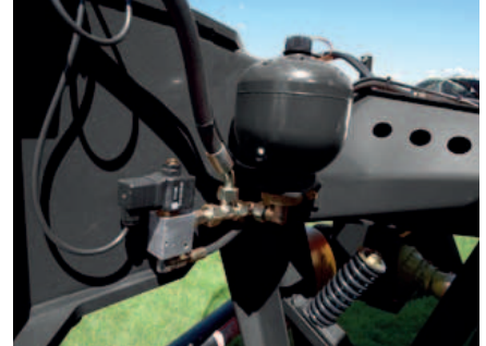
Hydraulic suspension ensures precise setting of ground pressure (EXTRA 440H).
